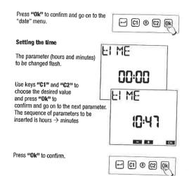
The instrument then goes into normal operational status and is ready for use. The display shows the values for the date, time, status relay 1, status relay 2 (when present), day of the week (on the first line in letters and lower down in numbers) and the GMT/BST symbol.
