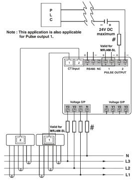
Pulse output from MRJ4M-SL meter can be interfaced into a process through a PLC for the on-line control of energy content in the process. If the PLC has a self exciting digital input, an external DC voltage supply is not needed.
