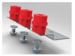
3) Fit the 20mm insulators to the direct connection mounting plate using the M6x6 screws/washers provided.
