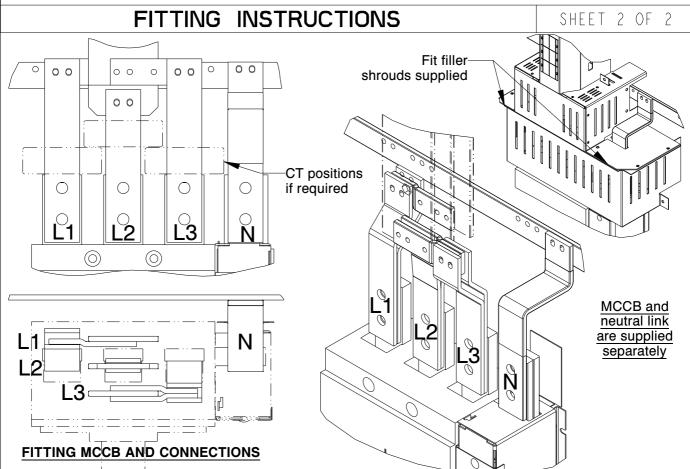
**NOTE:** When mounted above the panelboard, for top cable access, turn the unit upside down so that the MCCB mounting plate is closest to the busbars. Front plates can be refitted in their original orientation ie with louvres opening downwards.
