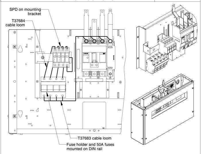
Unit is assumed mounted in accordance with the instructions supplied with the unit and the required MCCB is fitted
