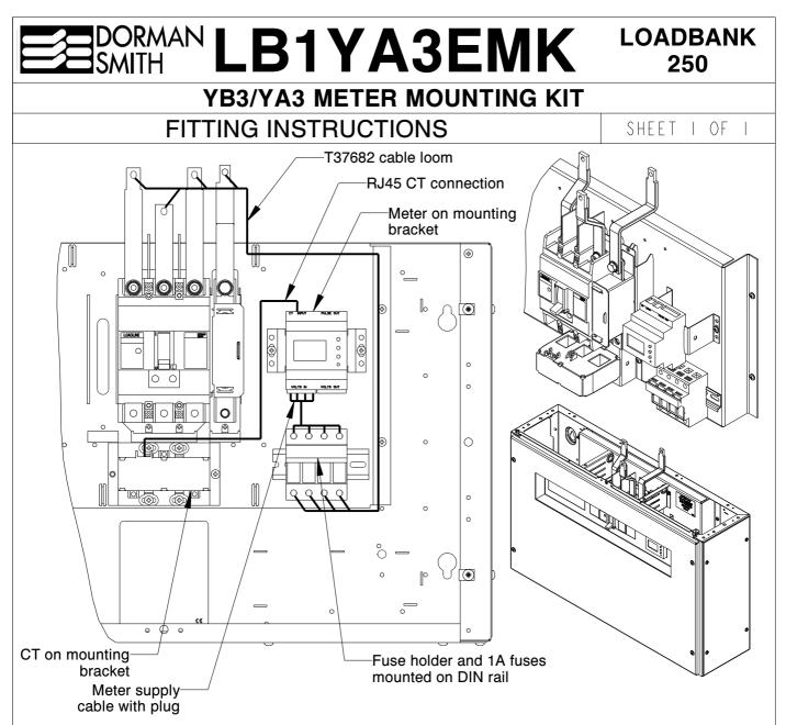
Unit is assumed mounted in accordance with the instructions supplied with the unit and the required MCCB is fitted.
