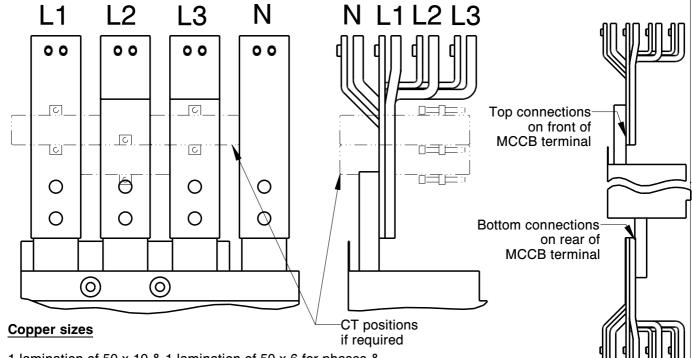
1 lamination of 50 x 10 & 1 lamination of 50 x 6 for phases & neutral
