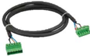
Meter to meter supply cable (1 off per additional meter) Meter knockouts are 120mm apart TAS-F-MTMSC0.30 - 0.3m long (for meters in adjacent knockouts) TAS-F-MTMSC0.50 - 0.5m long (for longer distances between meters) TAS-F-MTMSC1.00 - 1.0m long (for longer distances between meters)
