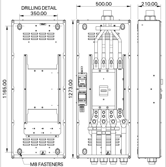
YA7 UNIT suitable for 2 x 4c 300mm cable or sc 630mm cable with Terminal Extension kit Cat No LLGPYA7EXT.
