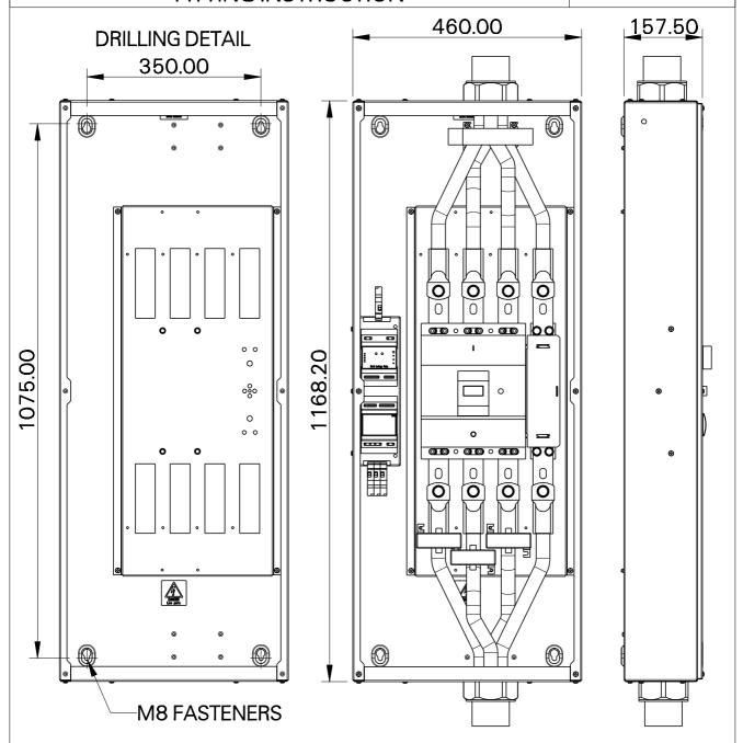
YA6 UNIT suitable for 4c 300mm cable using reduced palm cable lugs or 2 x 4c 185mm cable.
