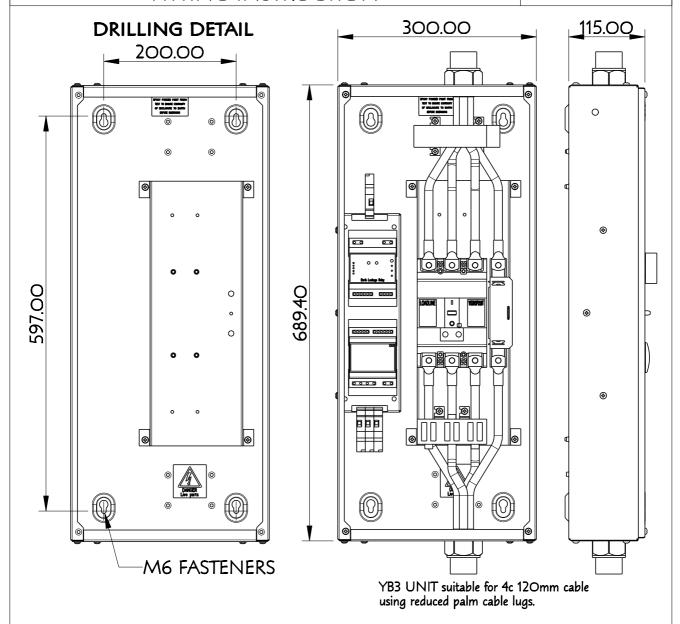
7: See MCCB instruction sheet for terminal screw torque values, on completion of cabling refit the end plates & front plate
