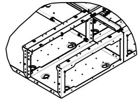
3 : If appropriate fit internal shield (B) between cableway and Loadbank
