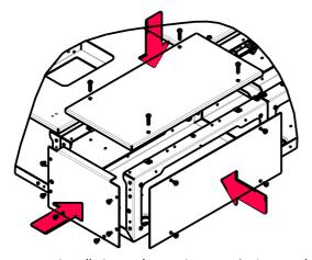
4: After installation of cables refit the front & end plates. using the thread forming screws provided in fastener kits. Reposition the side plate removed from the Loadbank unit on the side of the cableway as shown.
