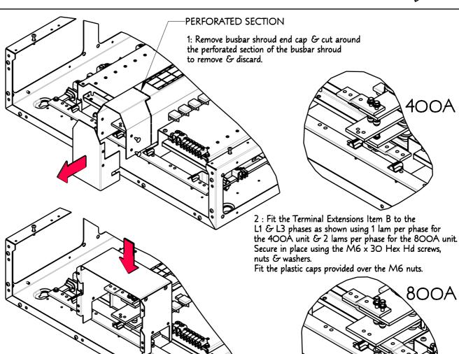
3: Fit Busbar End Shroud Item A over the terminals using the  $M5 \times 8$ self tapping screws provided.
