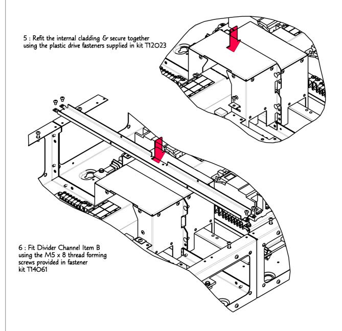
Connection screw recommended torque figure : M6 fasteners - 9Nm
