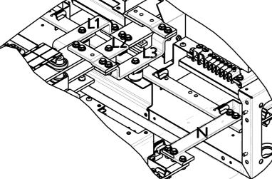
4 : Fit the L1 & L3 conns & packers as shown using the M6 x 20 Hex Hd screws, nuts & washers.
