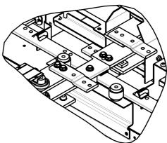
3 : Fit the L2 conn as shown using the M6  $\times$  20 Hex Hd screws, nuts & washers. Use an M6  $\times$  16 Hex Hd screw & washer to secure the conn to the support pillar.
